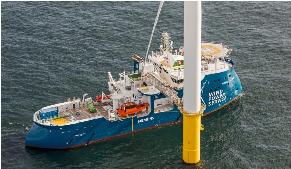
Figure 7-2: Offshore Wind SOV Performing Maintenance Activities (Credit: Ulstein)
