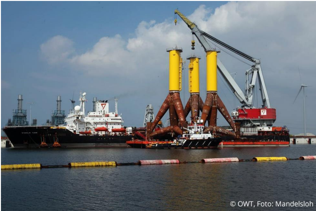
Figure 6-2: Tri-pod Foundations Ready to be Transported (Credit: Mandelsloh)
