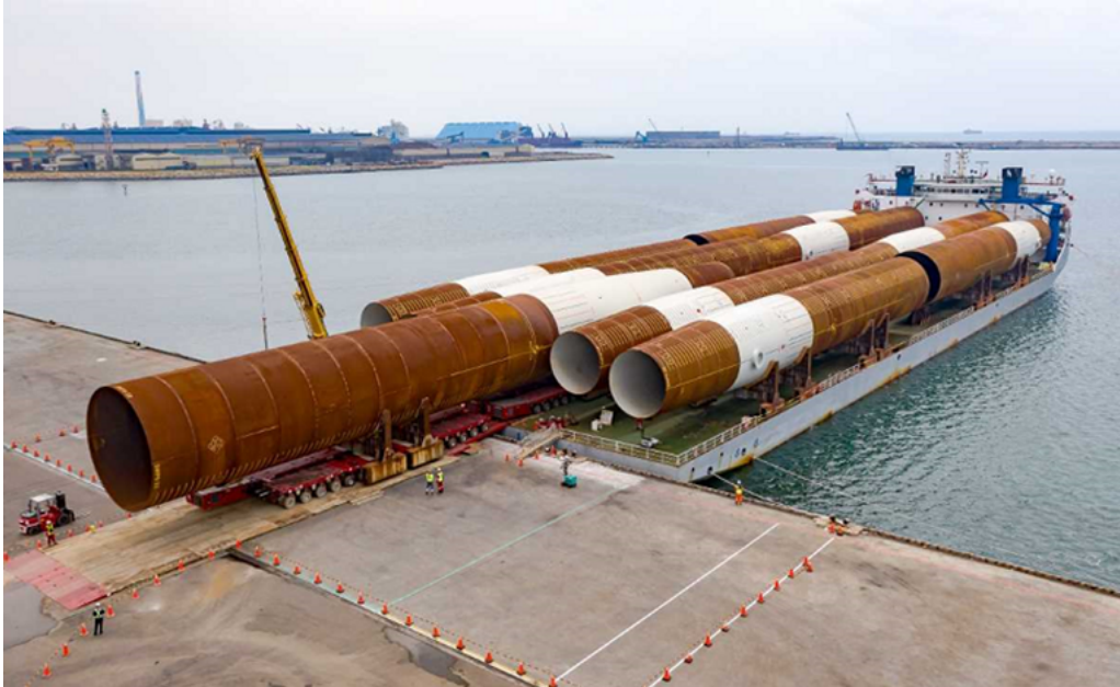
Figure 6-1: Monopile Foundations (Credit: ALE-Giant)
