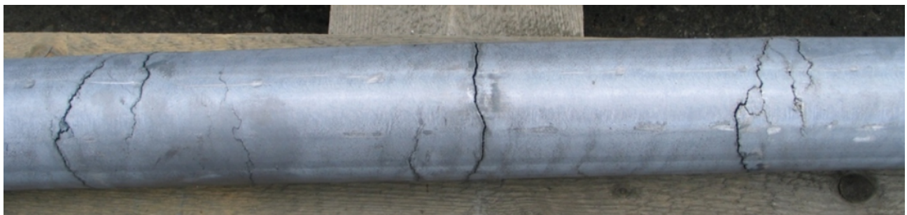
Figure 6-13: Lead Sheath Cracking from Fatigue Testing (Credit: ResearchGate - Björn Sonerud)
