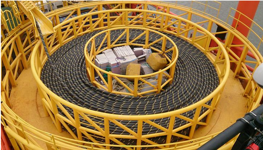
Figure 6-9: Cable Installation Vessel Carousel (Credit: Offshorewind.biz)
