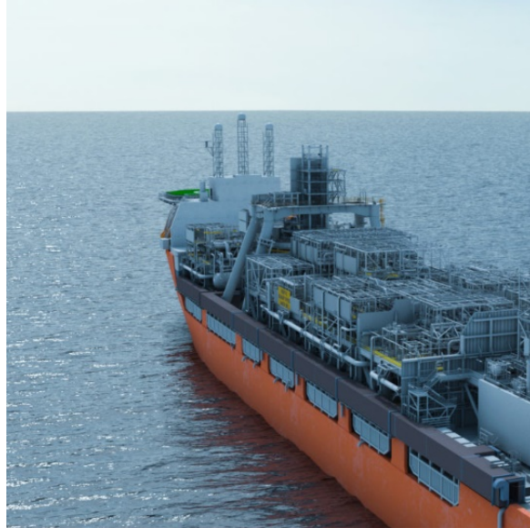
Figure 11-3 FPSO with CO 2 Capture
