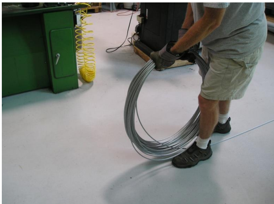
Picture 3-31: Unroll guy wires CORRECT
