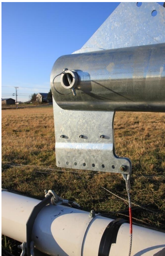
Picture 3-56: Lifter attachment to rocker plates
