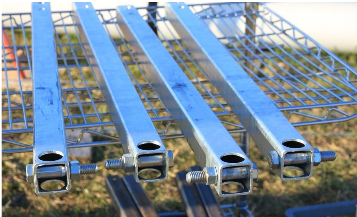
Picture 3-44: Install bolts/nuts onto jumper struts
