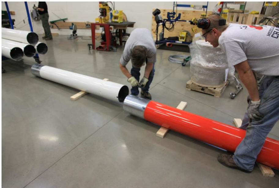
Picture 3-16: Attach tower bolt/nuts
