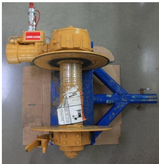
Picture 3-64: Super 60 Meter Bloom winch with mounting plate
