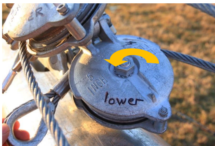
Picture 3-76: Reeving through pulley #4
