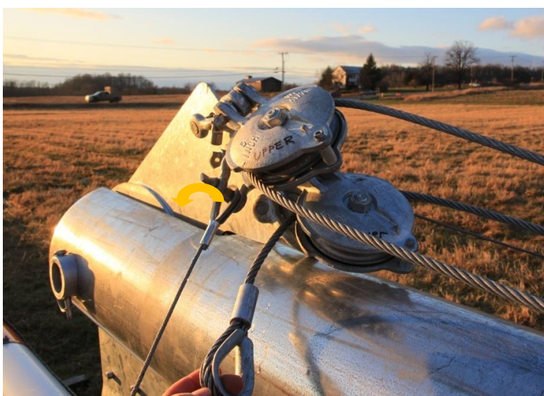
Picture 3-75: Reeving through pulley #4
