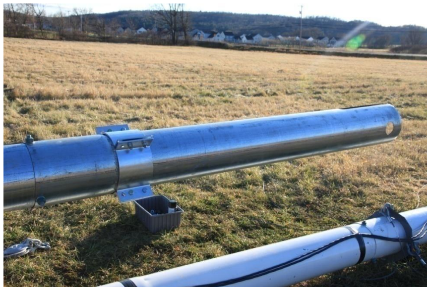
Picture 3-42: Ginpole jumper strut end-flange
