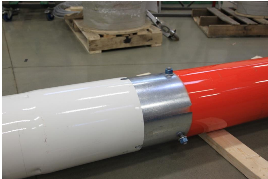
Picture 3-18: Sliding together tube sections
