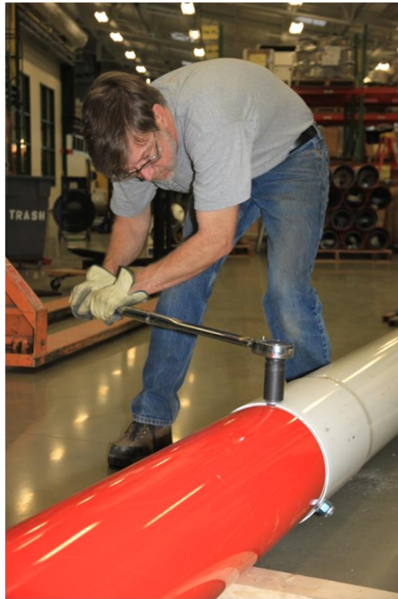
Picture 3-24: Torquing the nuts
