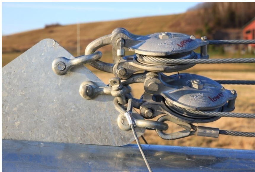
Picture 3-59: Correct block pulley assembly
