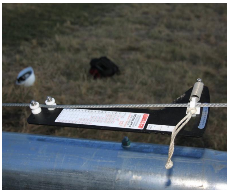
Picture 3- 80: Correct use of tension gauge
