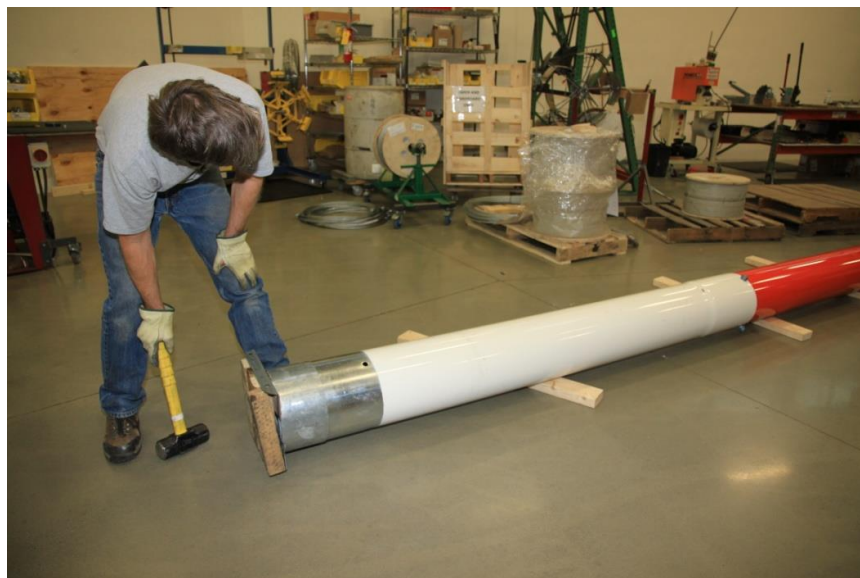
Picture 3-21: Seating the tubes with a mallet
