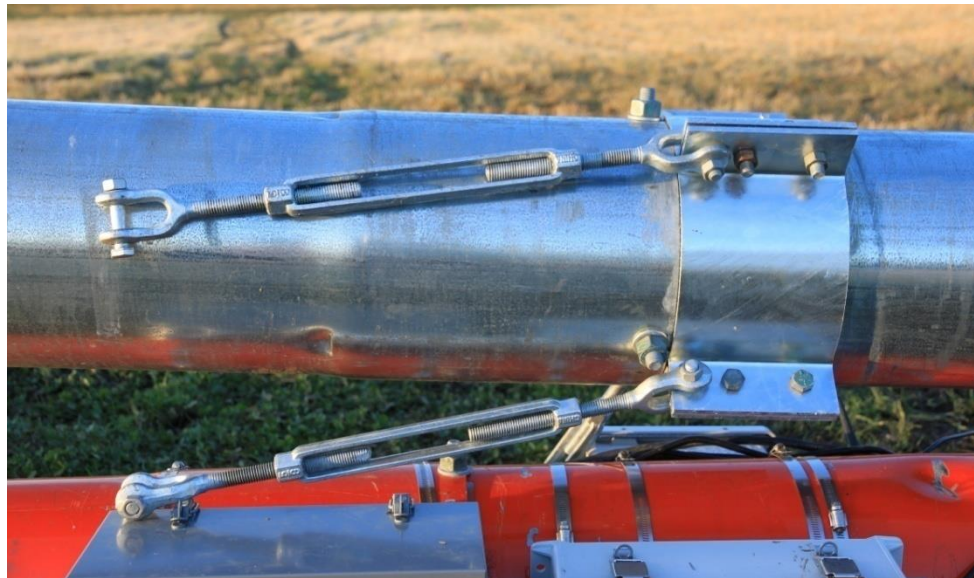
Picture 3-43: Turnbuckle assembly
