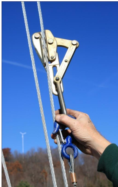
Picture 4-11: Using a Chicago grip
