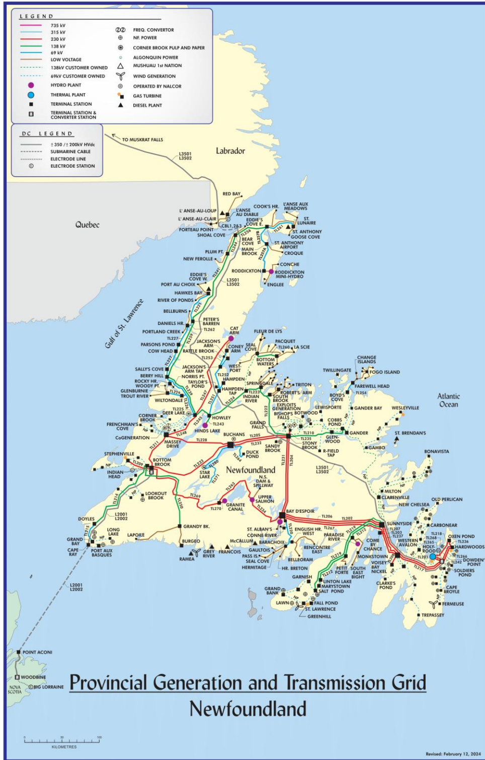
Figure 14 Detailed view of the transmission and generation assets that make up electricity system in Newfoundland
