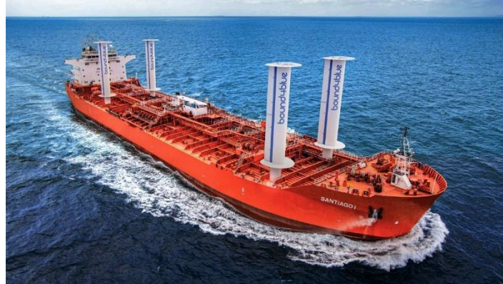
Figure 4: Example of an oil and chemical tanker utilizing suction sails 36 .
