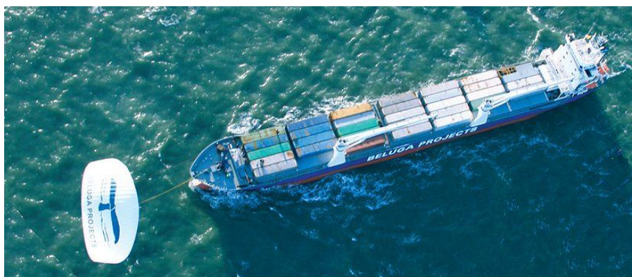
Figure 7: Example of a cargo vessel utilizing a kite 39 .
