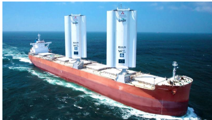
Figure 5: Example of a bulk cargo carrier utilizing wing sails 37 .
