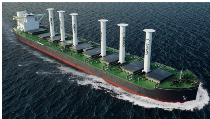
Figure 3: Example of a bulk carrier utilizing rotor sails 35 .
