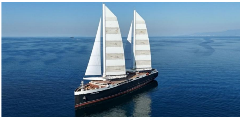
Figure 6: Example of a cargo vessel utilizing soft sails 38 .
